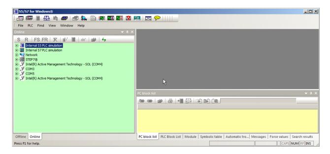
Expanding the appropriate port the MPI Bus will be scanned, and all stations will appear – in this case two stations were found.
