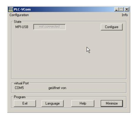
Select Configuration in the top Left corner, and select the PLC-VCOM option from the drop down menu.
