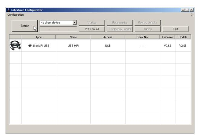
Once the adapter is found; select it, press the **Parameterize** button, and select the **Bus Configuration** option from the subsequent dialog.
