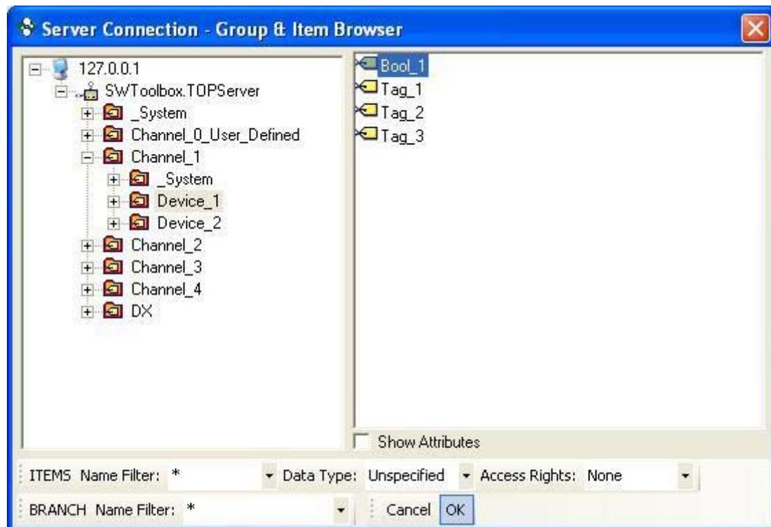
10. Now you must specify a condition and a value. We want this trigger to fire when the value of Bool\_1 is equal to False. After specifying a condition and value click OK. We have just added and configured the second Monitored Item Trigger.
