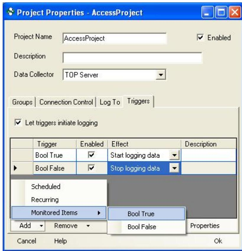
For this example we have enabled *Let triggers initiate logging*. With this option enabled once Start Logging is selected the project will only start logging data when the Bool True trigger fires. With this option disabled the project will start logging data as soon as Start Logging is selected.
