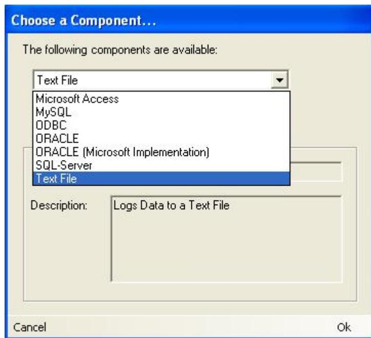
The Data Logger supports logging to Text files, Microsoft Access databases, MySQL databases, SQL Server databases, Oracle databases and ODBC databases. For more information about each Data Storage option please refer to the [Data Storage](#) section.
