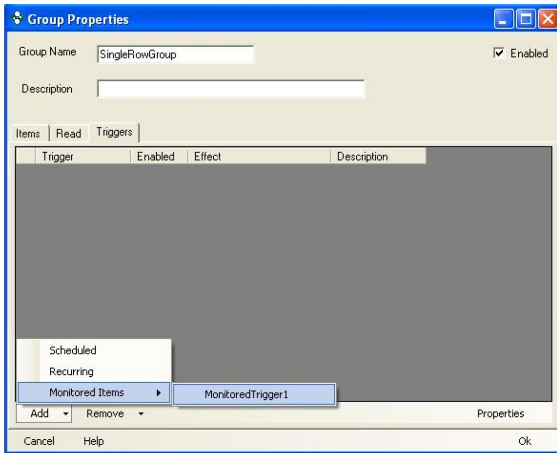
12. Now you must set the Effect the trigger will have. We want to set the effect to One-shot Read Now. Also make sure the enabled box is checked. You can now click Ok on the group properties and then select Ok on the project properties.
