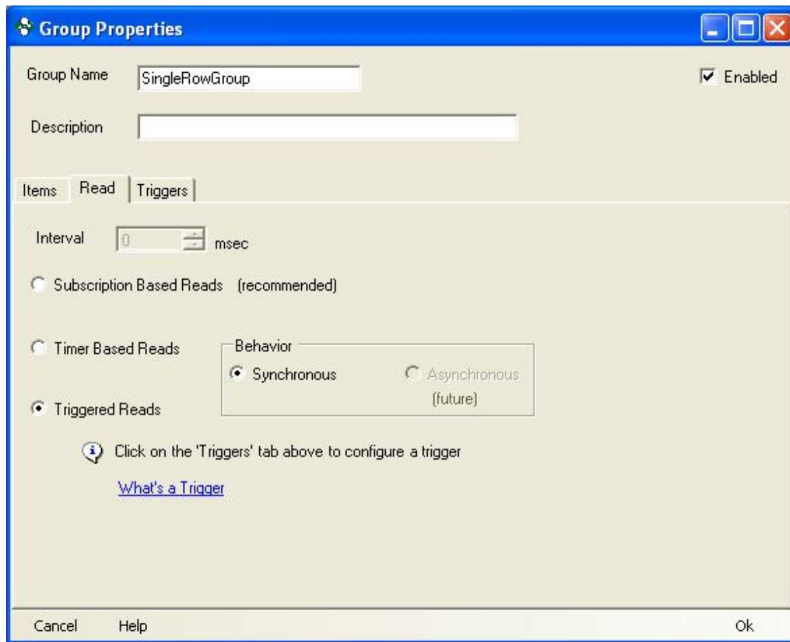
4. For this example we are going to be using a Monitored Item Trigger. To add a monitored item trigger right click on the Triggers icon in the tree view and select Add -> Monitored Item Trigger.
