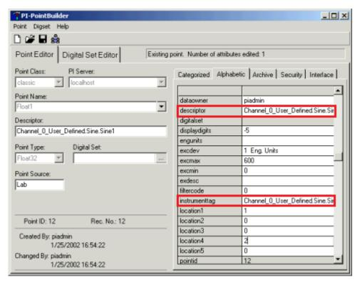
In **location1** enter any number, for the interface instance number – make note of this number, as it will be required later. If the number in **location1** does not match the number configured (later) in the OPCint.bat file, then the tag will be ignored.
