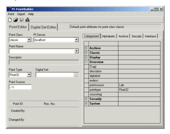
Assign the point a name in the **(Tag)** field, and the **Pointsource** should be changed to "O" to designate this as an OPC Connection. All tags definied in the PI Database that will be used by the OPC Interface must share a common point source.
