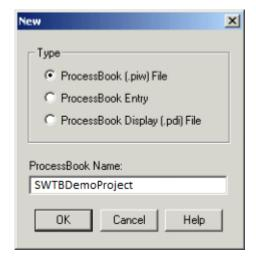
Select *OK*, and – in the new ProcessBook – navigate to **Insert | Display** to show show the new display dialog. In **Define ProcessBook Entry**, give the display a name, and select *OK* to finish – "Trend\_Example" is used in this example:
