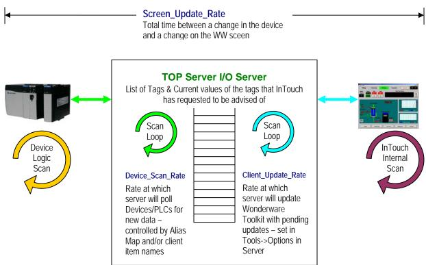
Note: simplifications have been made to this drawing for the sake of clarity about the key points we wish to make in this application note.
