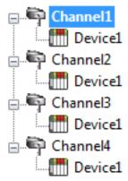
Each device can be defined under its own channel. In this configuration, a single path of execution is dedicated to the task of gathering data from each device. If the application has 256 or fewer devices, it can be optimized exactly how it is shown here.
