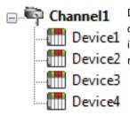
Devices appear under a single Aromat Ethernet channel. In this configuration, the driver must move from one device to the next as quickly as possible to gather information at an effective rate. As more devices are added or more information is requested from a single device, the overall update rate begins to suffer.
