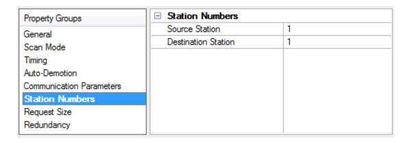
**Source Station**: Specify the station number that will identify the driver's connection point. Each node on the network must be assigned a unique station number. This includes the connection points in the driver (one per device object). Valid numbers range from 1 to 64, where 1 is the default. For more information, refer to ET-LAN Connection Properties.
