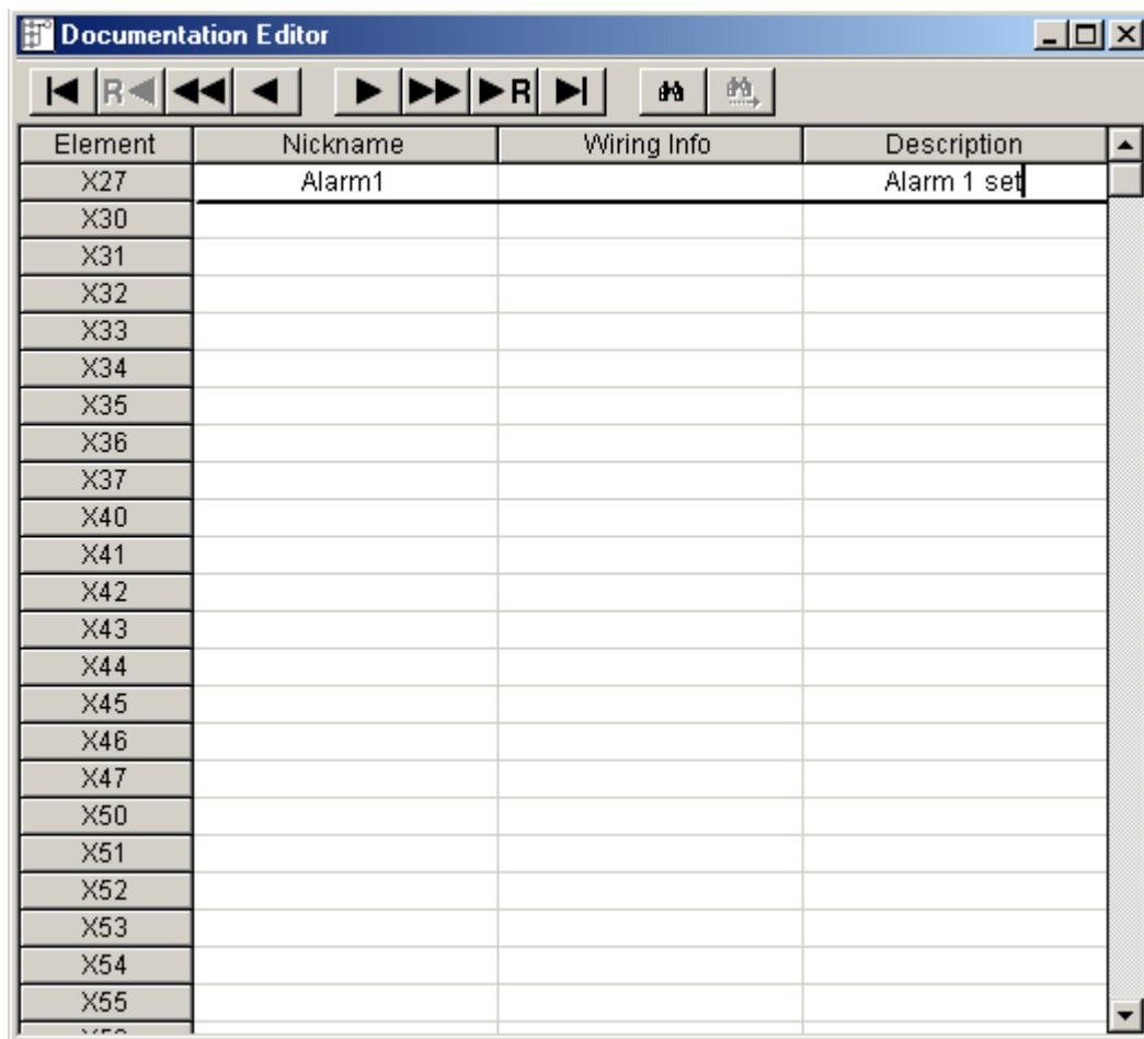
The screenshot shows the Documentation Editor window with a toolbar at the top and a table below. The table has four columns: Element, Nickname, Wiring Info, and Description. The 'Element' column lists memory references from X27 to X55. The 'Nickname' column contains 'Alarm1' for X27 and an empty cell for others. The 'Wiring Info' and 'Description' columns also contain empty cells. The 'Description' cell for X27 contains the text 'Alarm 1 set'.
