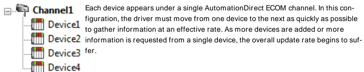
If the AutomationDirect ECOM Driver could only define one single channel, then the example shown above would be the only option available; however, the AutomationDirect ECOM Driver can define up to 100 channels. Using multiple channels distributes the data collection workload by simultaneously issuing multiple requests to the network. An example of how the same application may appear when configured using multiple channels to improve performance is shown below.
