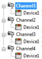
Each device can be defined under its own channel. In this configuration, a single path of execution is dedicated to the task of gathering data from each device. If the application has fewer devices, it can be optimized exactly how it is shown here.
