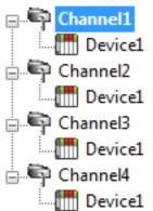
Each device can be defined under its own channel. In this configuration, a single path of execution is dedicated to the task of gathering data from each device. If the application has fewer devices, it can be optimized exactly how it is shown here.
