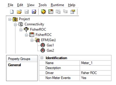
**Name**: This parameter specifies the meter name. Each meter must be assigned a unique name. The default setting is Meter\_n (where n increments up from 1 for the first meter).
