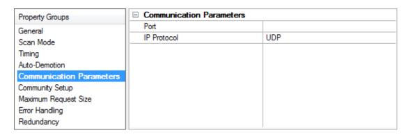
**Port Number**: This parameter specifies the port number that the remote device is configured to use. The default setting is 18901.
