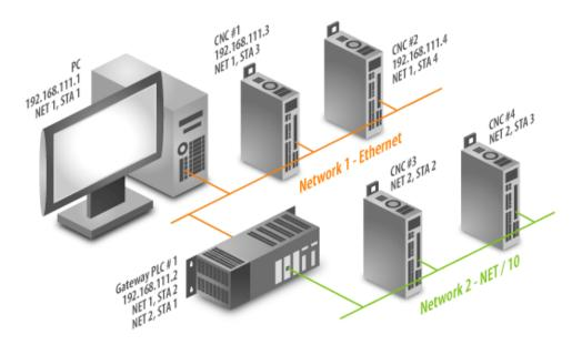
The gateway has an AJ/1QE71 Ethernet module and NET/10 module. CNC 1 and CNC 2 have an AJ/1QE71 Ethernet module and NET/10 module. CNC 3 and CNC 2 have a NET/10 module. In this example, four devices are created in the server project using the Device IDs listed in the table below.
