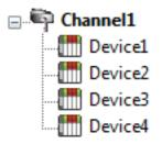
Channel1 Each device appears under a single device channel. In this configuration, the driver must move from one device to the next as quickly as possible to gather information at an effective rate. As more devices are added or more information is requested from a single device, the overall update rate begins to suffer.
