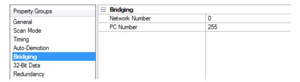
**Network Number**: This parameter specifies the Network Number of the target device. The valid range is 0 to 255, with 0 being used for local connections. The default setting is 0.
