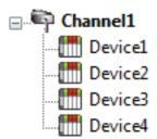
In this project, there is only one channel defined. All devices that need to be accessed are defined under that one channel. The Modbus Plus Driver must move from one device to the next as quickly as possible to gather information at an effective rate. As more devices are added or more information is requested from a single device, the update rate begins to suffer.
