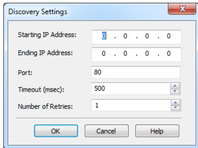
**Starting IP Address:** Specify the starting IP address. The default setting is 0.0.0.0.
