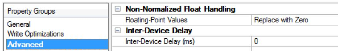
**Non-Normalized Float Handling:** A non-normalized value is defined as Infinity, Not-a-Number (NaN), or as a Denormalized Number. The default is Replace with Zero. Drivers that have native float handling may default to Unmodified. Non-normalized float handling allows users to specify how a driver handles non-normalized IEEE-754 floating point data. Descriptions of the options are as follows:
