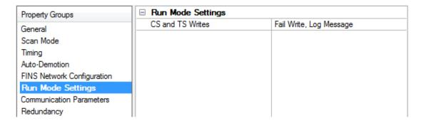
**CS and TS Writes**: Select how the device performs writes in Run mode. The default setting is Fail Write, Log Message.
