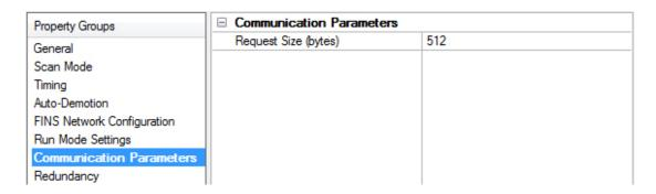
**Request Size**: This parameter specifies the maximum number of bytes that may be requested from a device at one time. The default setting is 512 bytes. To refine the driver's performance, set the request size to one of the following settings: 32, 64, 128, 256, 512, 1024, or 1984 bytes.
