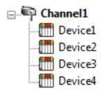
Devices appear under a single channel. In this configuration, the driver must move from one device to the next as quickly as possible to gather information at an effective rate. As more devices are added or more information is requested from a single device, the overall update rate begins to suffer.
