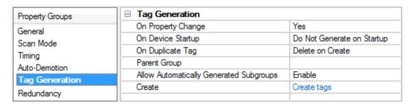
On Property Change: If the device supports automatic tag generation when certain properties change, the On Property Change option is shown. It is set to Yes by default, but it can be set to No to control over when tag generation is performed. In this case, the Create tags action must be manually invoked to perform tag generation. To invoke via the Configuration API service, access /config/v1/project/channels/{name}/devices/ {name}/services/TagGeneration.
