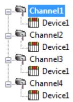
Each device can be defined under its own channel. In this configuration, a single path of execution is dedicated to the task of gathering data from each device. If the application has 100 devices, it can be optimized exactly how it is shown here.
