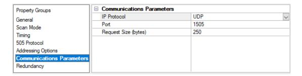
IP Protocol: This property specifies whether the driver should connect to the remote device using the User Datagram Protocol (UDP) or Transfer Control Protocol (TCP). This driver requires Winsock V1.1 or higher.
