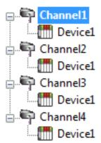
Each device can be defined under its own channel. In this configuration, a single path of execution is dedicated to the task of gathering data from each device. If the application has 100 or fewer devices, it can be optimized exactly how it is shown here.
