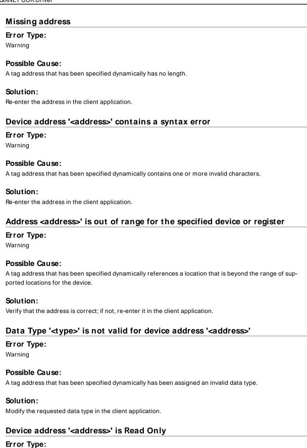
A tag address that has been specified dynamically has a requested access mode that is not compatible with what the device supports for that address.
