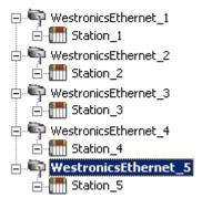
Each device can be defined under its own channel. In this configuration, a single path of execution is dedicated to the task of gathering data from each device. If the application has fewer channels, it can be optimized exactly how it is shown here.
