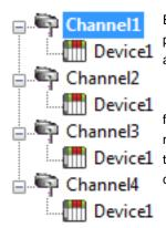
Each device can be defined under its own channel. In this configuration, a single path of execution is dedicated to the task of gathering data from each device. If the application has 32 or fewer devices, it can be optimized as it is shown here.
