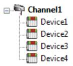
Each device appears under a single channel. In this configuration, the driver must move from one device to the next as quickly as possible to gather information at an effective rate. As more devices are added or more information is requested from a single device, the overall update rate begins to suffer.
