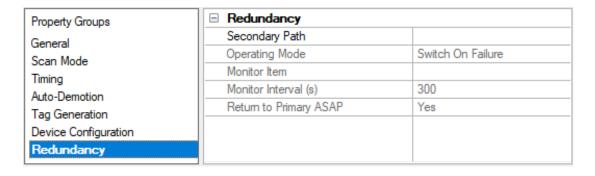
**Secondary Path**: Specifies the explicit, unaliased path to the device serving as backup if the primary device fails. The valid format is <channel>.<Device>.
