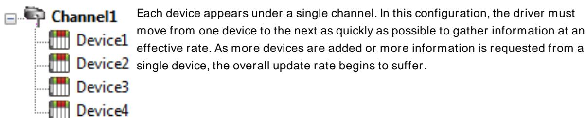
If the Yokogawa MX Driver could only define one single channel, then the example shown above would be the only option available; however, the Yokogawa MX Driver can define up to 100 channels. Using multiple channels distributes the data collection workload by simultaneously issuing multiple requests to the network. An example of how the same application may appear when configured using multiple channels to improve performance is shown below.
