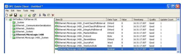
10. Next, go online with the MicroLogix and display both Channel 1 – Ext Channel Status and the B3 Data File. Toggle bit B3:0/0 once and you should see Number of events to be reported increment to 1 and then go back to zero after five seconds. You should also see Trans Unsolicited Res FC Counter increment by 1, as well as Received Confirm FC Counter:
