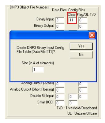
2. Word B11:0 now defines the Class (1, 2 or 3) for Binary Inputs 0-15. We will assign these Binary Inputs to Class 1 by setting the value of B11:0 to 1:
