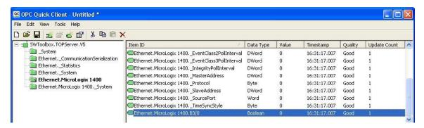
3. Because we gave the tag address an Explicit sub-type, TOP Server is reading this specific binary input once a second. We can see the read command initiated by TOP Server and the response from the MicroLogix in the following Wireshark Ethernet packet captures:
